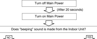
Check the voltage of power(About AC 115V, 60Hz)
